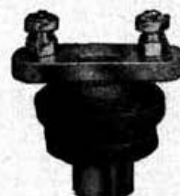
EDDYSTONE All-Wave H.F. Choke. Low loss D.L.-9 former with two section honeycomb wound coils. One screw fixing. Wavering 12.5 to 2,000 metres. Self capacity 2.4 m.mfd. Inductance 17.9 millihenries. D.C. resistance 60 ohms. No. 1066 ... 2/3
