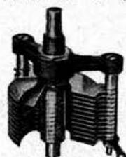
EDDYSTONE New Type Microdensers with improved D.L.-9 Insulation. No. 1094. 18 m.mfd. high-voltage type. Minimum, 3 m.mfd. Maximum, 18 m.mfd. D.C. flash-over voltage, 3,500 volts ... 4/3 No. 1129. 40 m.mfd. high-voltage type. Minimum, 3.8 m.mfd. Maximum, 40 m.mfd. D.C. flash-over, 2,300 volts 4/9 No. 1093. 60 m.mfd. high-voltage type. Minimum, 4 m.mfd. Maximum, 59.5 m.mfd. D.C. flash-over, 2,300 volts. 4/11 No. 1131. 160 m.mfd. Minimum, 4.75 m.mfd. Maximum, 161 m.mfd. D.C. flash-over voltage, 1,000 volts ... 6/6
